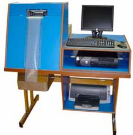
**Harmonic Analysis:** Our new software module for the FILMTEST can calculate and represent graphically the fundamental wave and the high harmonics of a thickness profile.
